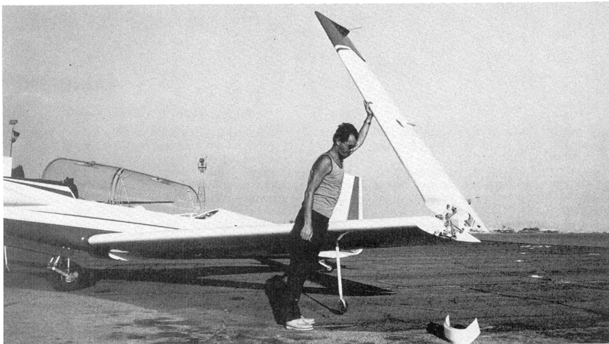
Charles M. Gyenes, vice president of Aerosport, shows how to shorten almost 60-foot wingspan to less than 37 feet for hangaring. Ailerons align automatically when wings are extended and locked.
