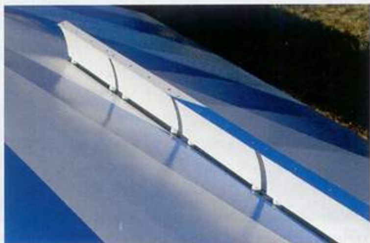
Cruising at 100 kt gives four hours endurance. Below: 35 hp Rectimo VW engine. Spoilers are an essential landing aid.
