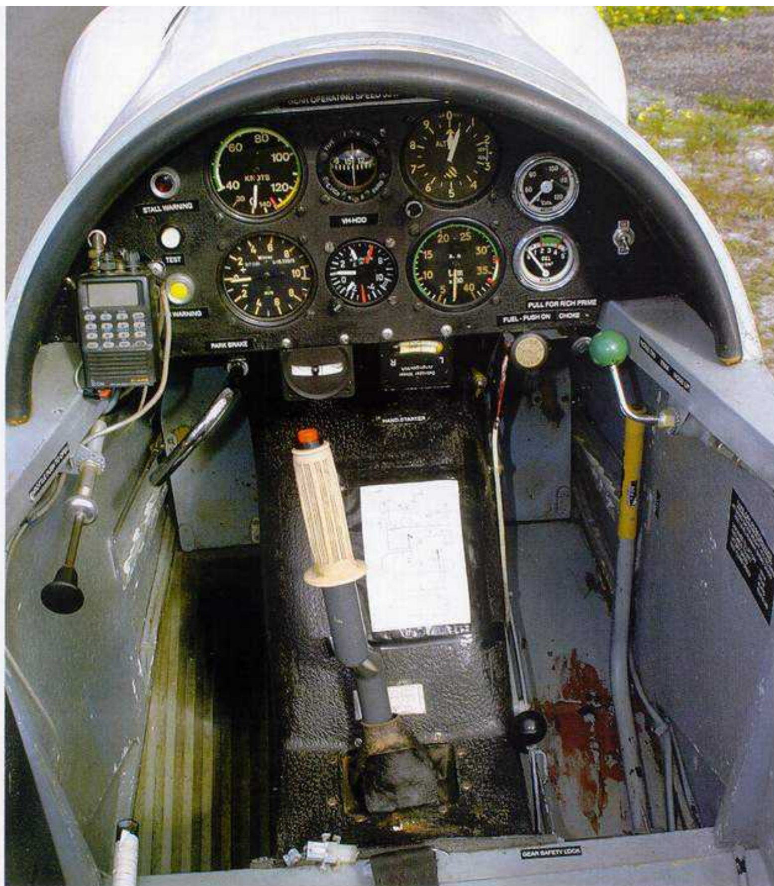
Cockpit has undercarriage lever on the right, spoiler extender on the left, recoil starter, centre right, handbrake and throttle on left. Note separate upright and inverted slip ball, g-meter.
