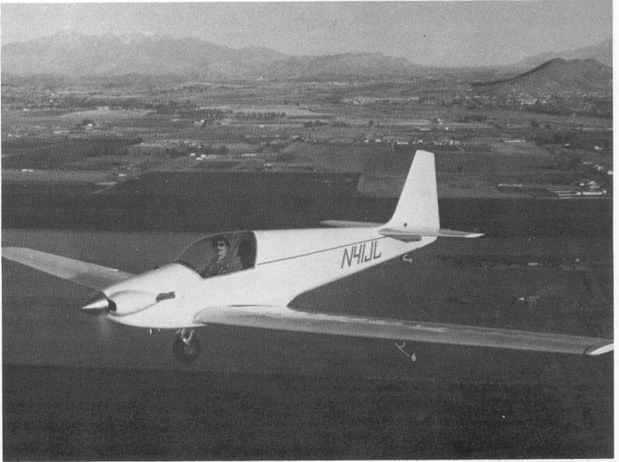
An airborne author, in his favorite airplane. Sleek little RF-4D shows its retractable landing wheel in the extended position.
