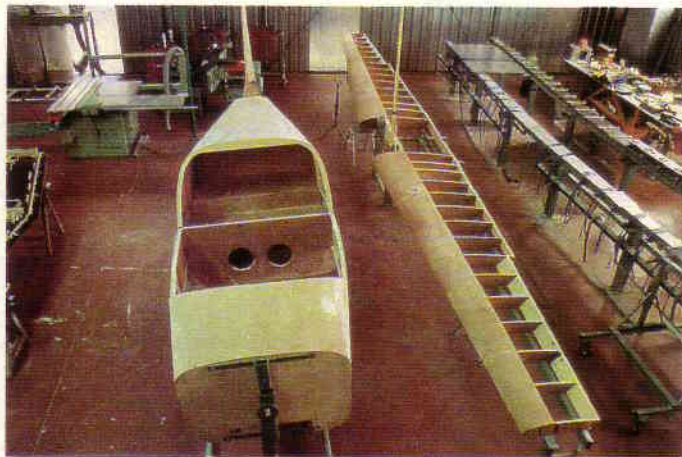
Opposite: the RF-47 is very obviously a Fournier design. Above: René Fournier in the cockpit of the prototype. Below: the second prototype under construction at Tours, using a new wood/carbon fibre composite which requires no autoclave.
