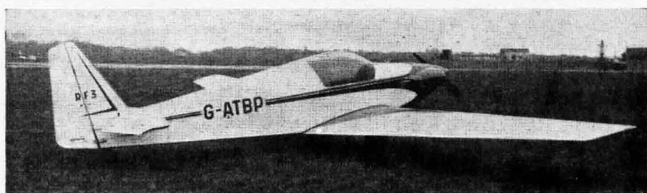
The R.F.3 used in this test. The tip skids have been fitted with roller-skate wheels to ease taxi-ing on hard runways (Photos: "Air Pictorial")
